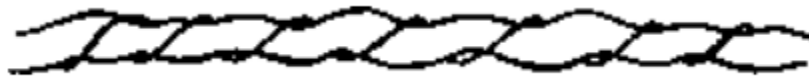
(b) SPIRA or GIMP- combination of soft, thick yarns twisted with fine, hard yarns
